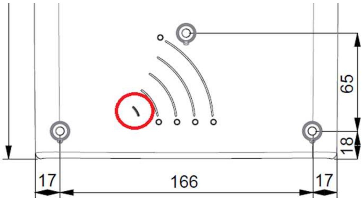
Figure 3 Location of capacitive sensor
